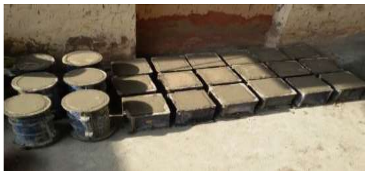
Fig. 2: Casting of Cubes and cylinders
