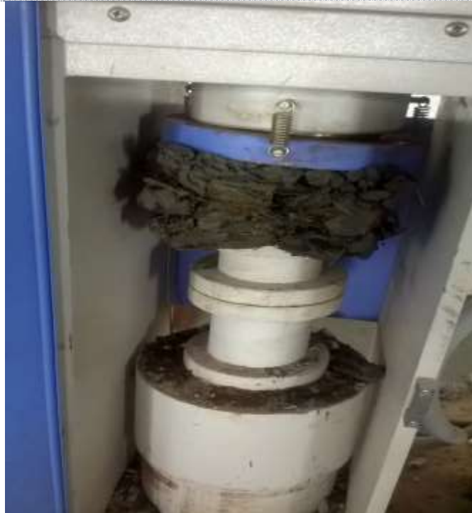
Fig. 5: cube after compressive load
