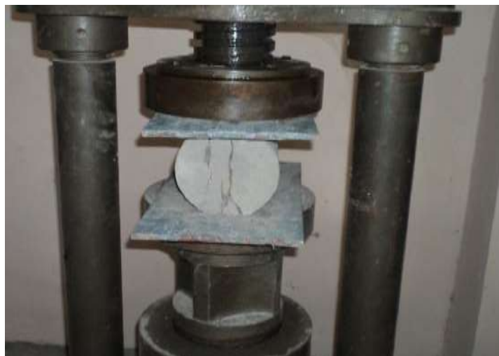
Fig. 6: Specimen loading for split tensile strength test
